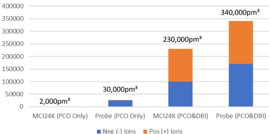
Tests were conducted for BLS by GreenTech in 02/2017 utilizing an ion meter placed 3' from the downstream side of each unit. Units used were the MCI22K and the MCI™ SynAIRgPure probe with a NO O<sub>3</sub> producing PCO cell.
