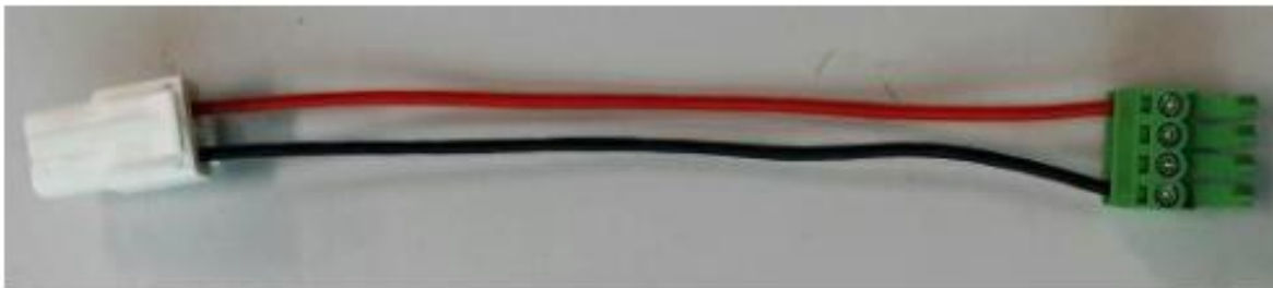
Line and connector for power connection with FCU
