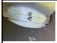
3) The screw on the opposite side of the molex will secure the support bracket to the base of the probe.
